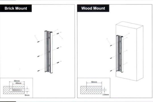
Put Screw Cover and Metal Shelf on Aluminum Support, use the screw drive to tighten the bolts, put on plastic covers
