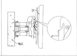
There is a bolt under both of the left and right brackets, screw out a majority of the bolts before mounting, and re-screw down them to against closely to the wall plate after the brackets have been hung firmly.
