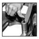
2 To adjust the tilt angle of your display, have one person hold the display firmly in place while another person loosens the tilt adjustment knobs located on either side of the mount (see illustration). Once the knobs are loose you can move the display to the desired angle. Tighten the knobs securely before releasing the display.
