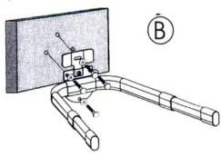
3. Push the plastic cover onto the bracket.
