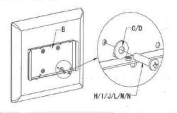
Step4: Hang the TV fixed plate in connection with the TV panel on the wall dead plate.
