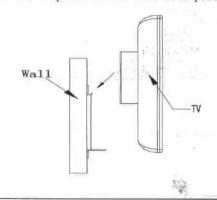
Step5: Screw down two bolts under the wall fixed installation for the panel TV.
