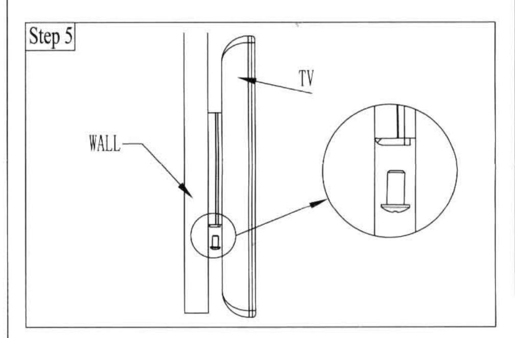
Step 5: Screw down four bolts under the wall fixed installation for the panel TV.
