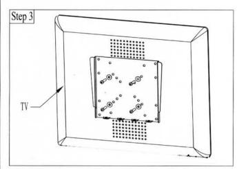
Step 3: Install TV fixed plate on the TV back. Select four suitable bolts from the parts bag and screw them into the bolt-holes in the back of the TV.
