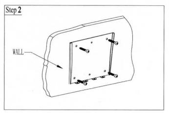
Step 2: Screw four lag bolts into the plastic concrete anchors through the wall dead plate to make the dead plate and vertical wall into a whole.
