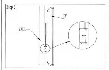
Step 5: Screw down four bolts under the wall fixed installation for the panel TV
