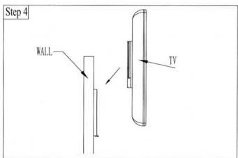
Step 4: Hang the TV fixed plate in connection with the TV panel on the wall dead plate.
