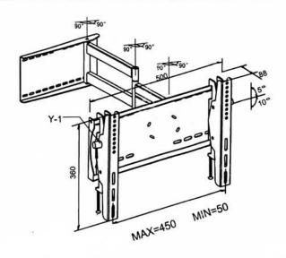
1. The viewing angle of plasma can be adjusted by loosen or tighten Y-1.
